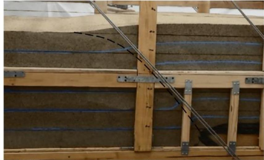
Figure 44: 12.44 cm of basal displacement beneath loose virgin sand. The dotted line represents the rupture plane. The edges have been cropped for clarity.
